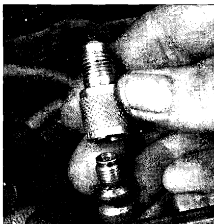
A typical high side adapter fitting like this must be used with the General Motors post-1976 type (3/8-24 thread) high side service valve before the hose can be attached
