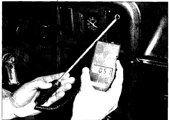
The best place to check the output of the evaporator is at the dash vent nearest the evaporator (usually one of the center vents)
