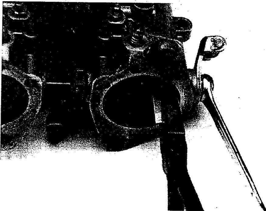
caused by the sealing arrangement no longer keeping out moisture so that corrosion ruins the bearing. If the bearings have to be replaced, before starting this procedure make sure that you have new butterfly screws, nuts and locking washers on hand as well as the parts to be replaced (spindle or bearings or both).
