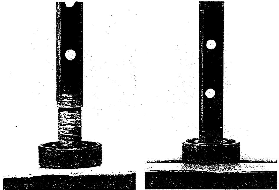
Photos show a spindle being tapped into a new bearing. Use a copper hammer or an aluminum drift to tap the spindle into the bearing. The spindle is guided to a large degree, but do make sure the spindle is square to the bearing and that the bearing is placed flat on the top of the vice jaws. Lubricate the bearing bore and spindle.
