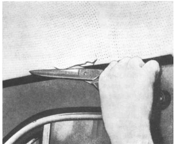
Fig. 72. Cutting away the headlining
