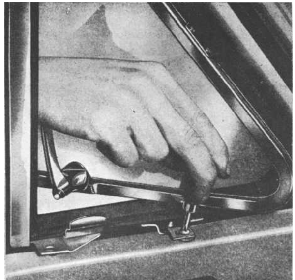
Fig. 30. Attaching screw for ventilation window
