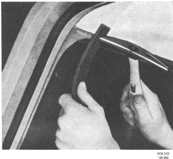
Fig. 45. Adjusting teazel strip
