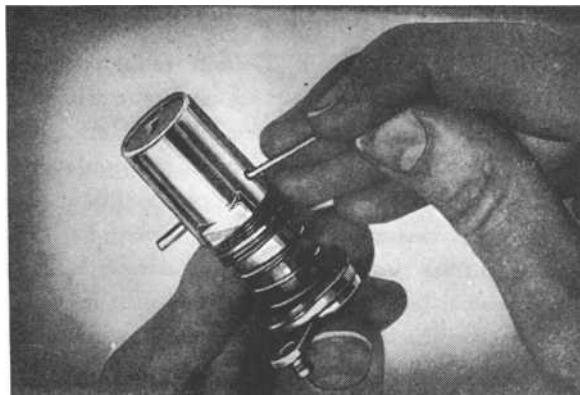
Fig. 24. Pressing out the locking pin
