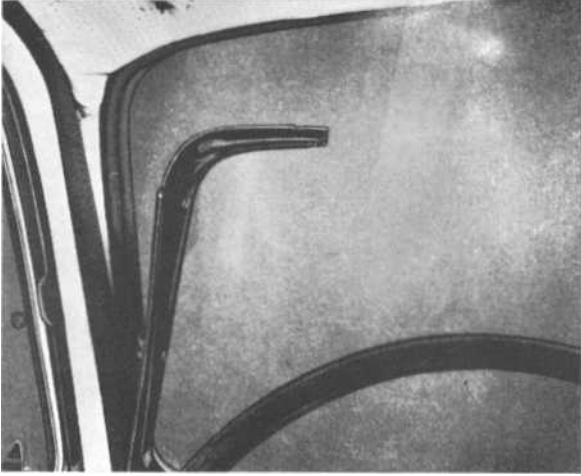
Fig. 67. Inner trim mouldings removed
