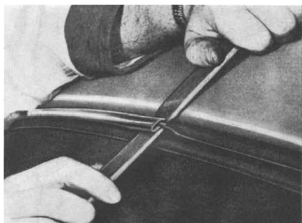
Fig. 54. Removing trim moulding from rubber strip
