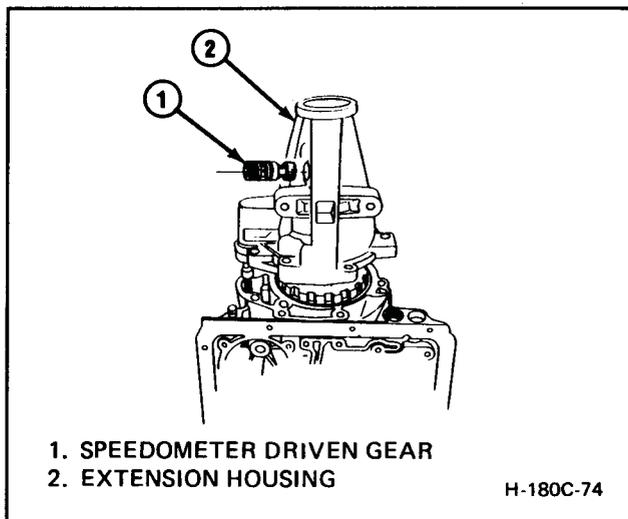
Figure 180C-76 Extension Housing and Speedometer Driven Gear
