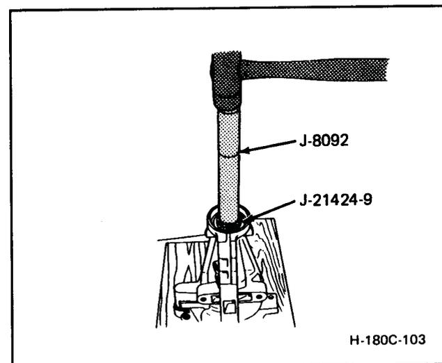
Figure 180C-103 Removing or Installing Extension Housing Bushing
