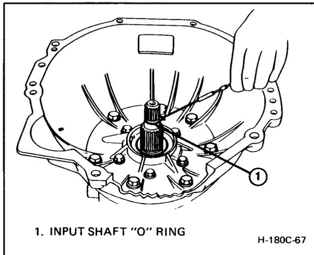
Figure 180C-70 Installing "O" Ring Seal on Input Shaft
