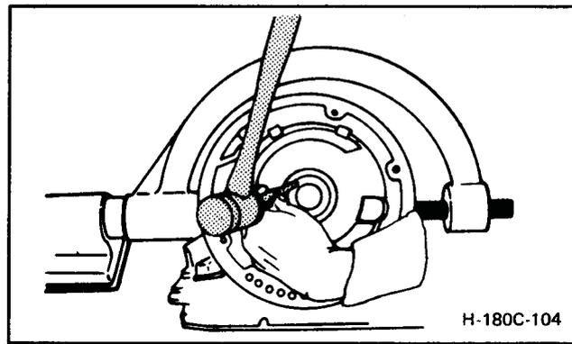
Figure 180C-105 Removing Reaction Sun Gear Drum Bushing Sleeve
