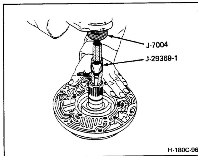
Figure 180C-96 Removing Oil Pump Bushing - Front
