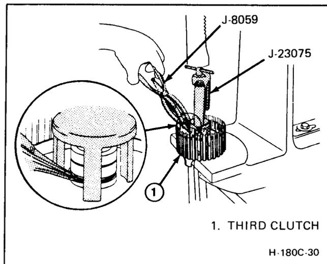
Figure 180C-41 Removing or Installing Third Clutch Piston
