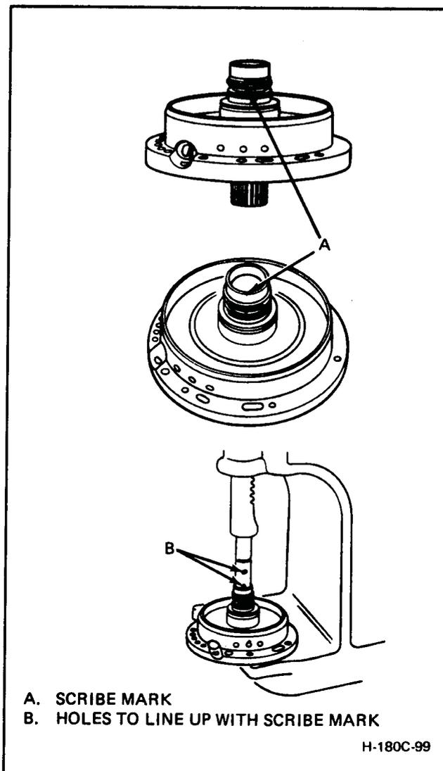
Figure 180C-99 Installing Oil Pump Bushing - Rear (Inner)
