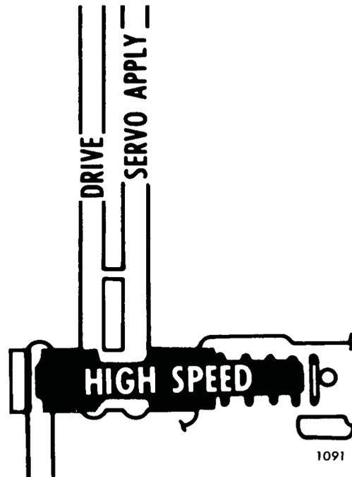
When a 3-2 shift is forced at high speed, the application of the band must be delayed. Servo apply pressure is directed through the high speed downshift timing valve.
