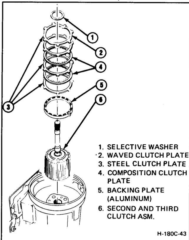
Figure 180C-55 Installing Second/Third Clutch Assemblies Into Case
