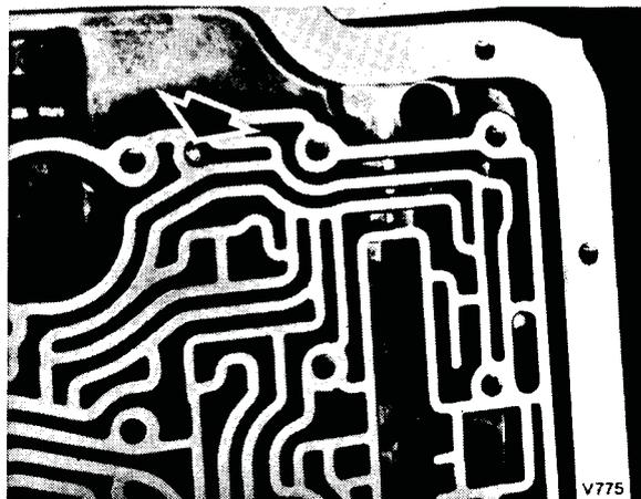
Later models use the following transfer plate identification numbers: 30 for 1759 cm<sup>3</sup> engine; 31 for 2279 cm<sup>3</sup> engine; 15 for the GM 2,1 litre diesel engine; 33 for Cavalier with a 16S engine and 22 for Cavalier with a 19S engine. The transfer plate of some early Cavalier models with the 16S engine are identified by 6V-notches.
