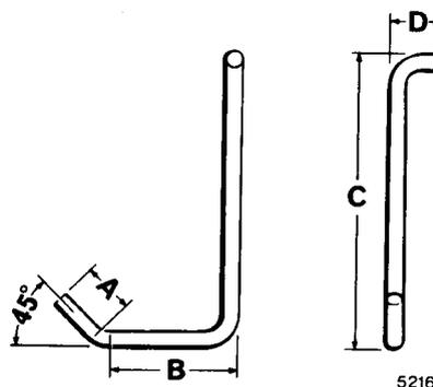
Depress one end of retaining ring out of groove in clutch drum and use hook to hold ring in this position.
