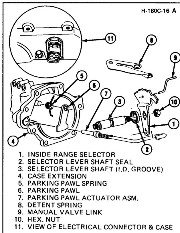
Figure 180C-34 Selector Lever Assembly and Electrical Connector
