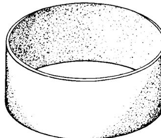
THE T-1082 COMPRESSES THE SECOND CLUTCH PISTON SEAL AND THEN GUIDES IT INTO ITS BORE. IF THIS TOOL WERE NOT UTILIZED, DAMAGE TO THE PISTON SEAL COULD RESULT.
