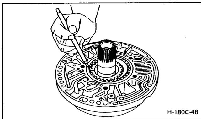
Figure 180C-59 Marking Location of Oil Pump Gear
