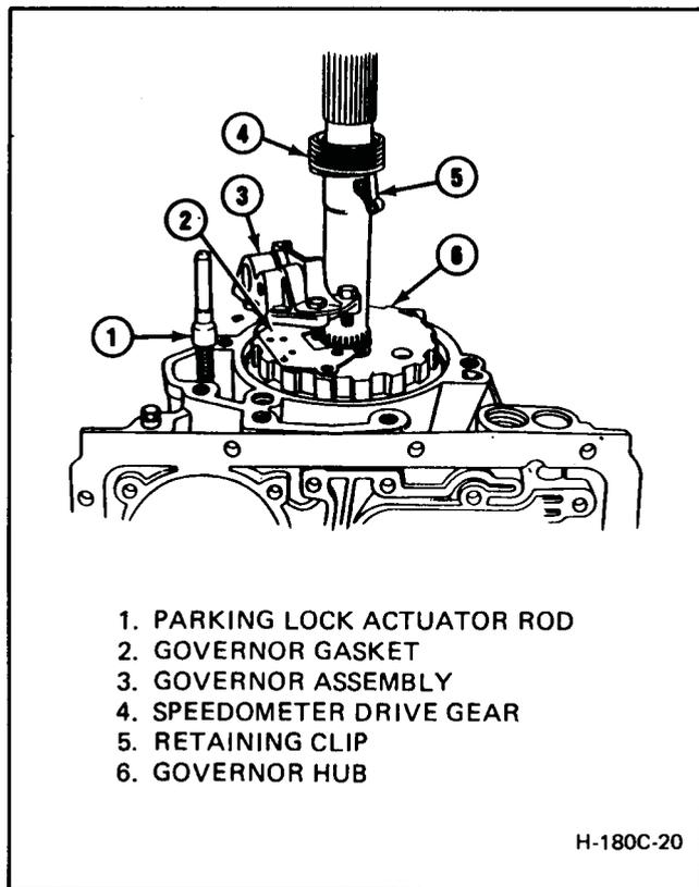
Figure 180C-73 Installing Governor Body and Speedometer Drive Gear
