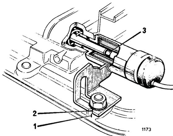
3. On models with a solenoid place a 0.25 in. diameter steel ball (3) inside solenoid and temporarily install into transmission case. Holding solenoid in position make a mark (1) on transmission case in line with notch (2) on mounting bracket.
