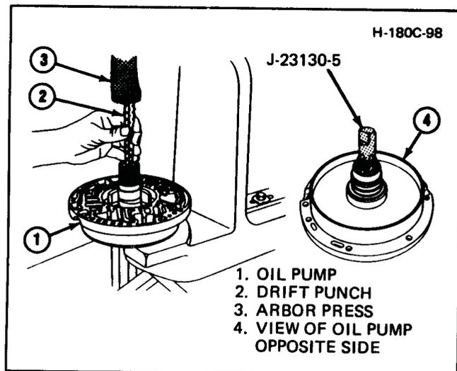
Figure 180C-98 Removing Oil Pump Bushing - Rear (Inner)
