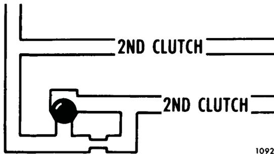
For reasons of shift timing it is necessary to have different restricting orifice sizes for the feed and exhaust of the second clutch. This is accomplished by introducing a check ball in the second clutch circuit.
