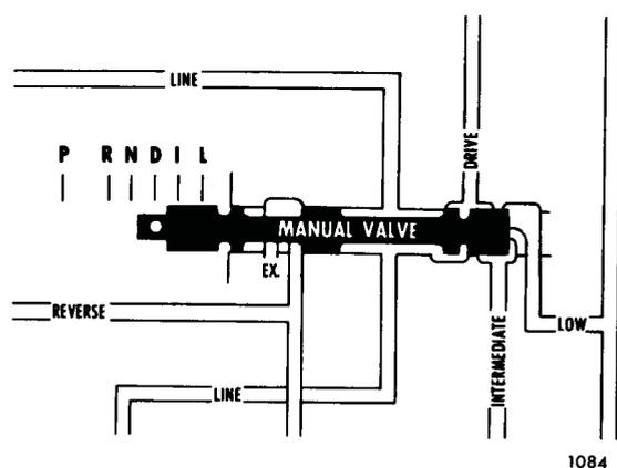
The manual valve is mechanically connected to the selector lever. Its function is to direct hydraulic pressure to the various circuits to establish the base hydraulic range of the transmission.
