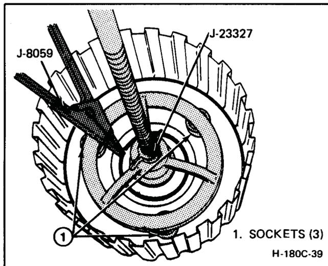
Figure 180C-50 Removing Snap Ring from Second Clutch Piston
