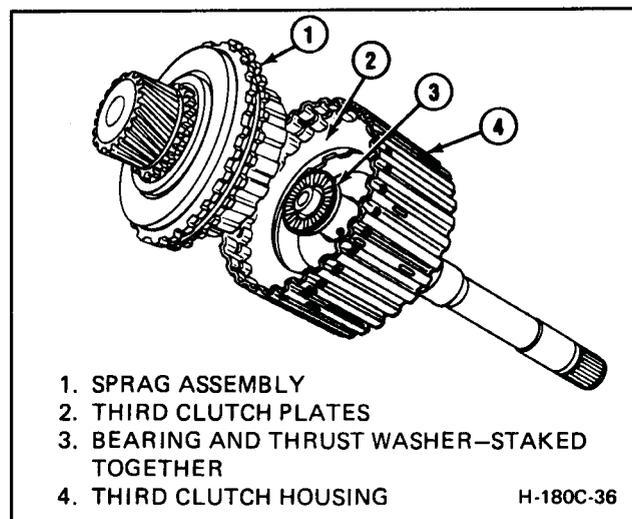
Figure 180C-47 Installing Sprag Assembly Into Third Clutch Assembly
