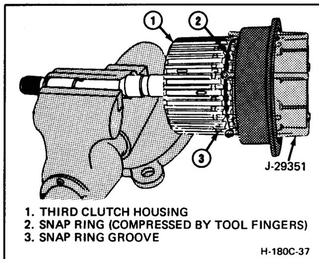
Figure 180C-48 Installing Retaining Ring in Third Clutch
