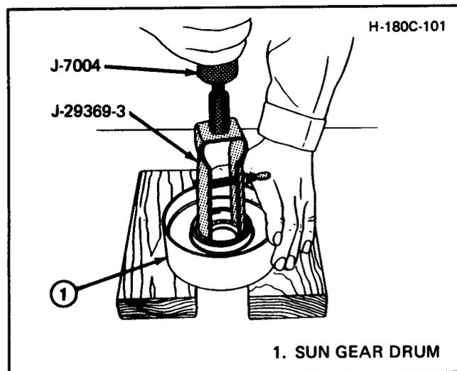
Figure 180C-101 Removing Reaction Sun Gear Drum Bushing
