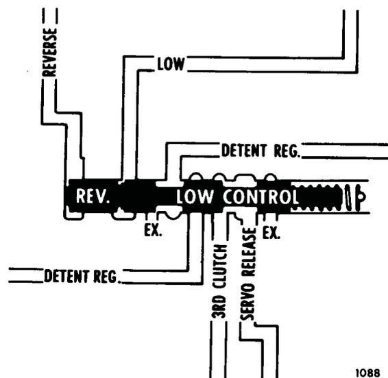
When the selector lever is placed in 'reverse', line pressure acts on the end of the reverse control valve and forces the low control valve into the same position as in 'low'. This causes the third clutch to be applied.
