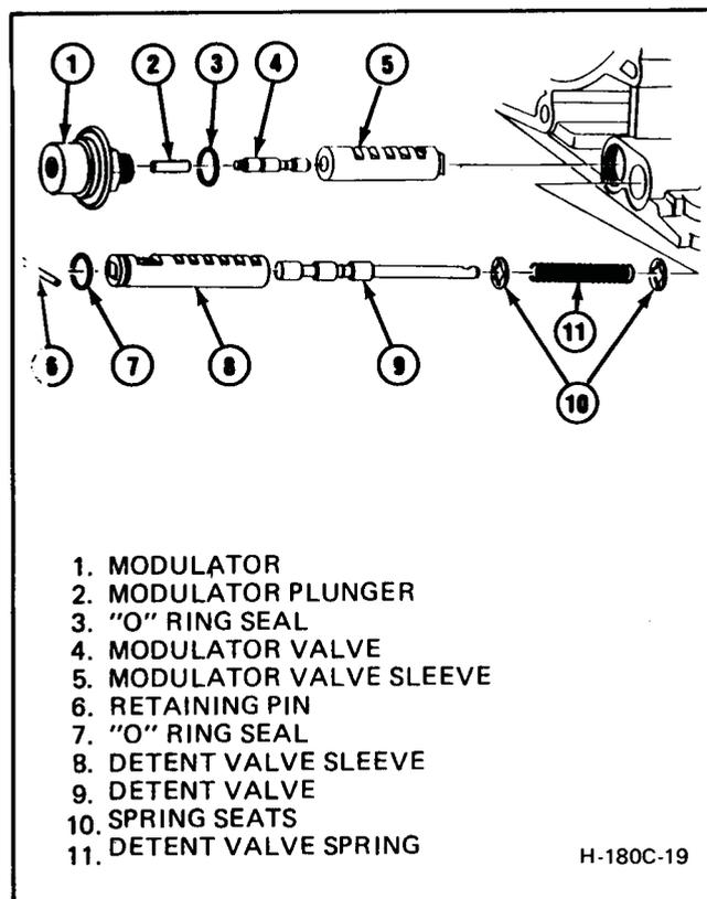
Figure 180C-77 Installing Detent Valve and Modulator Valve
