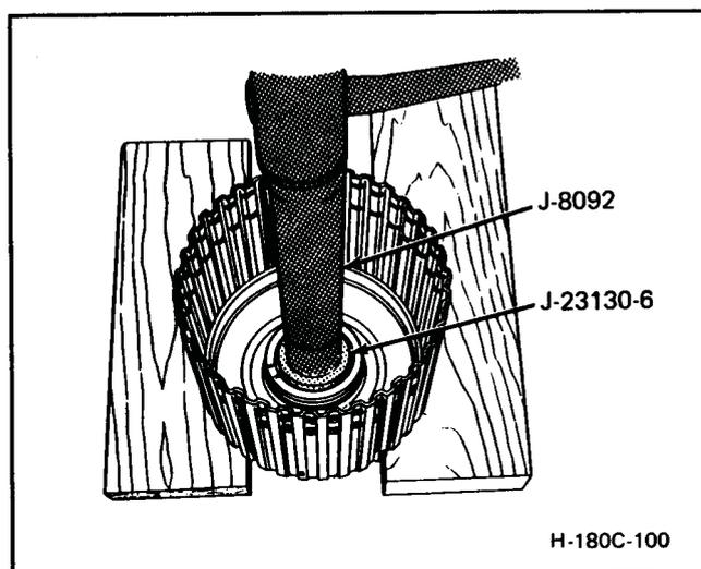
Figure 180C-100 Removing or Installing Second Clutch Bushing
