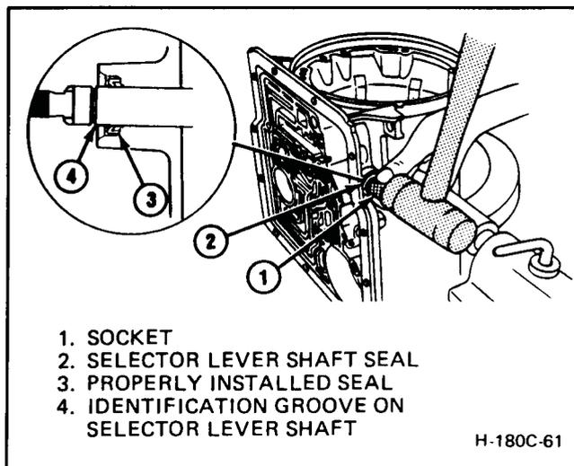
Figure 180C-33 Selector Lever Shaft Oil Seal Installation
