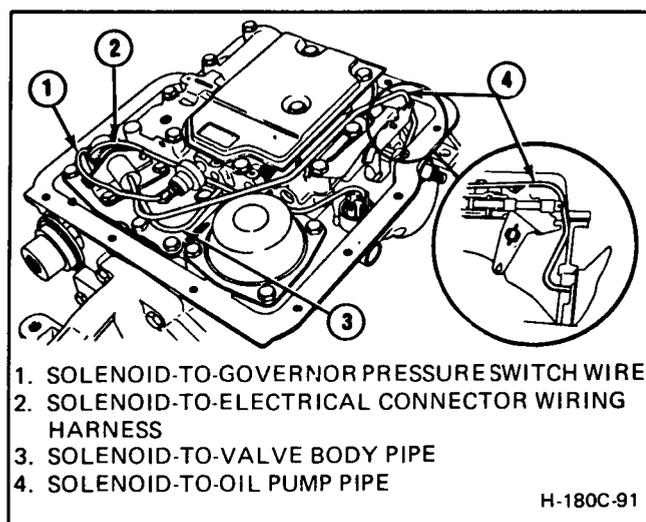
Figure 180C-91 Hookup of Solenoid Pipes and Electrical Wires
