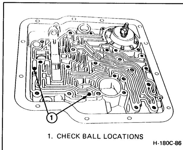
Figure 180C-88 Installing Check Balls in Oil Passages
