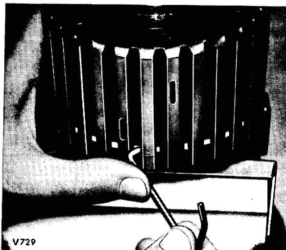
Using a small screwdriver, continue to depress retaining ring out of groove in clutch drum while at the same time applying a direct upward load on input shaft. This prevents the retaining ring from jumping back into its groove. Remove wire hook and withdraw clutch drum and input shaft assembly from sprag clutch.
