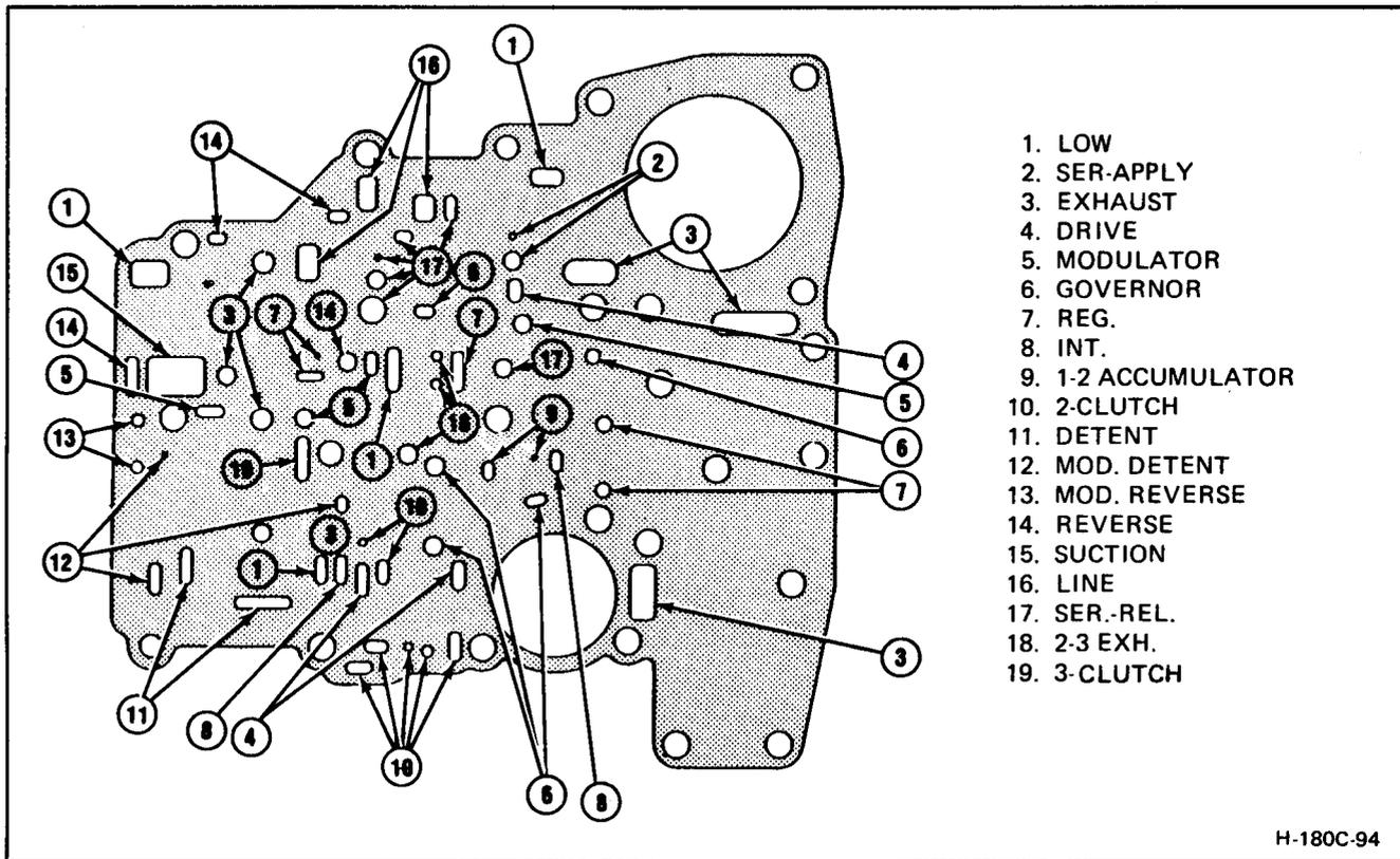
Figure 180C-17 Valve Body Transfer Plate Oil Passages
