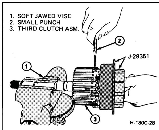
Figure 180C-29 Removing Third Clutch Retaining Ring
