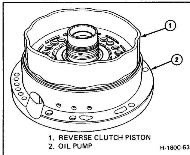
Figure 180C-63 Installing Reverse Clutch Piston Into Oil Pump
