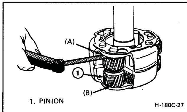
Figure 180C-28 Planetary Carrier and Pinion Clearance
