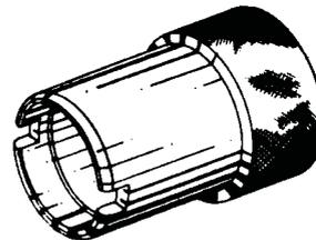
TO PREVENT EXCESSIVE WEAR TO THE FRONT SEAL AND BEARINGS, IT IS NECESSARY TO MAKE SURE THERE IS NO MISALIGNMENT BETWEEN THE CONVERTER HOUSING AND TRANSMISSION CASE. THE T-1080 CAN ALSO BE USED TO CHECK THE CLEARANCES IN THE FRONT PUMP. REFER TO SERVICE MANUAL.
