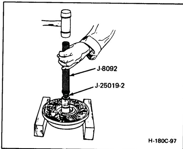
Figure 180C-97 Installing Oil Pump Bushing - Front
