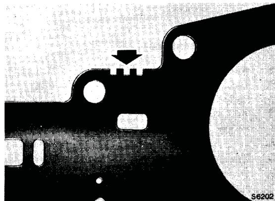
On four-cylinder models a revised transfer plate is also used with the revised valve body. The revised transfer plate can be identified by the number 12 on models with a 1256 cm<sup>3</sup> engine, three square notches on models with a 1759 cm<sup>3</sup> engine and one square notch on models with a 2279 cm<sup>3</sup> engine.
