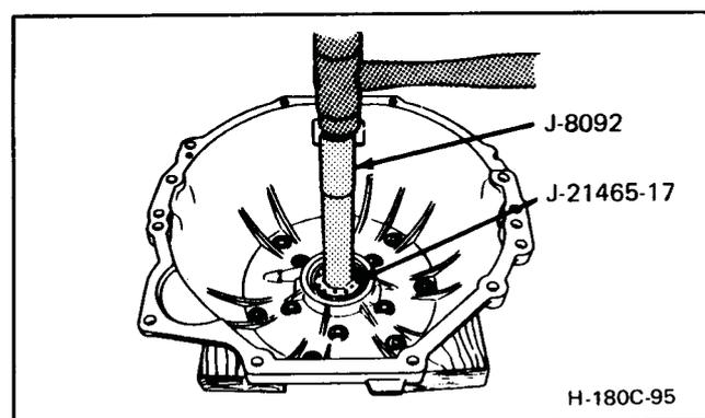
Figure 180C-95 Removing or Installing Converter Housing Bushing
