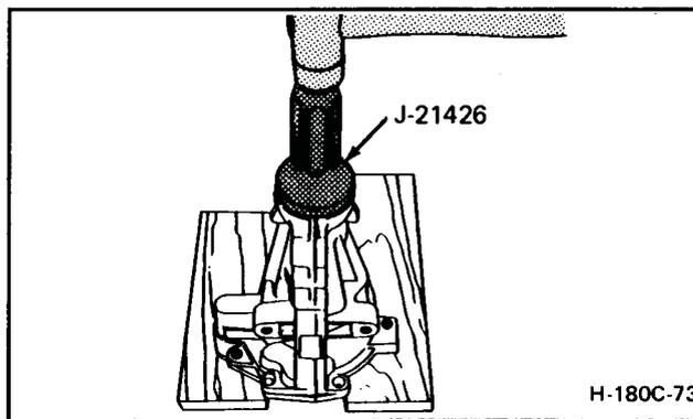
Figure 180C-75 Installing Extension Housing Oil Seal
