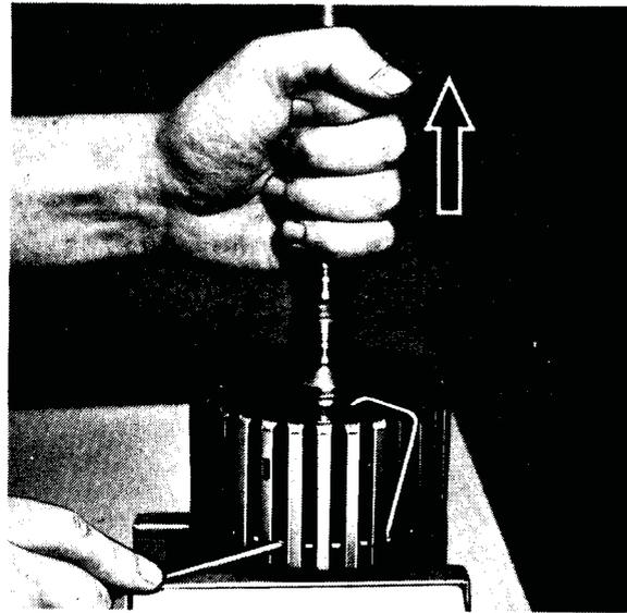
When reassembling, use screwdriver to compress retaining ring while simultaneously pressing down on the sprag clutch race.
