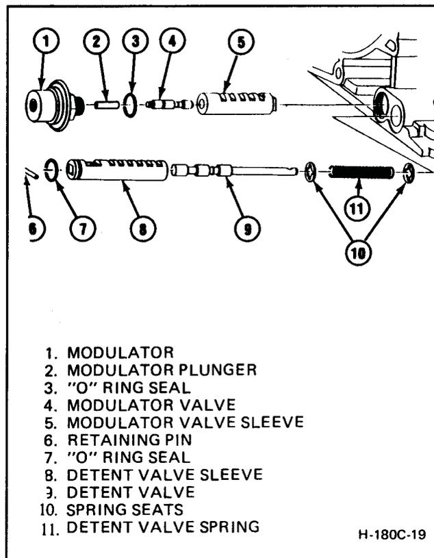
Figure 180C-25 Modulator and Detent Valve Assemblies
