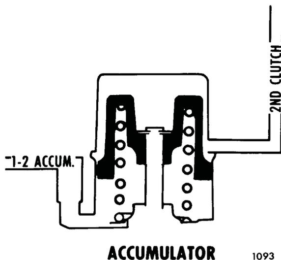
In order to obtain a smooth 1-2 upshift, it is necessary to control the rate of pressure build-up on the second clutch piston. This is accomplished by introducing a hydraulic modulator into the clutch circuit.
