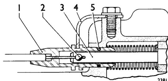
6. On models with a cable-operated detent valve, rear cable (1) is a push fit into the transmission case after locating inner cable (2) into the detent valve (3). The cable is retained by a bracket (4). Oil leakage is prevented by a rubber O-ring (5).
